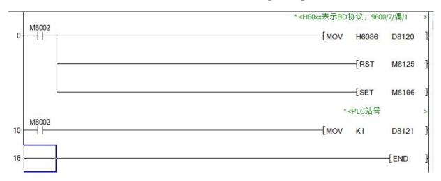
The touch screen sets the BD protocol master station, that is, it can communicate with the PLC.
